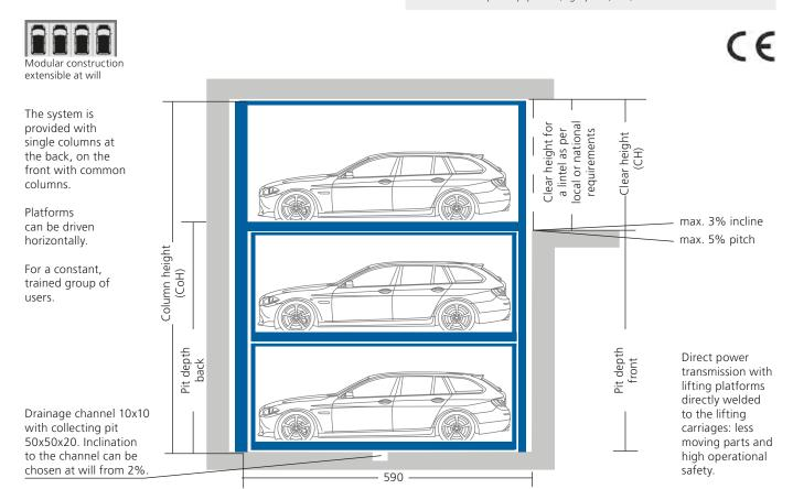
Standard system length 590 cm for vehicles with a max. length of 500 cm and a max. weight of 2.000 kg. Platforms for different vehicle length or higher vehicle weight could have impact on the system length! Further dimensions, inclusive for drive-through systems, available upon request.
