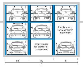
System dimensions for vehicles with a max. weight of 2.000 kg. Platforms for higher vehicle weight could have impact on system dimensions! Further dimensions, inclusive for drive-through systems, available upon request.
