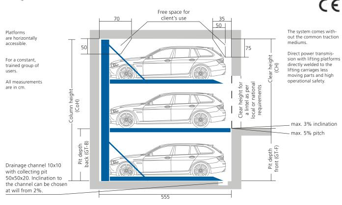
Standard system length 555 cm for vehicles with a max. length of 500 cm and a max. weight of 2.000 kg. Platforms for different vehicle length or higher vehicle weight could have impact on the system length! Further dimensions, inclusive for drive-through systems, available upon request.
